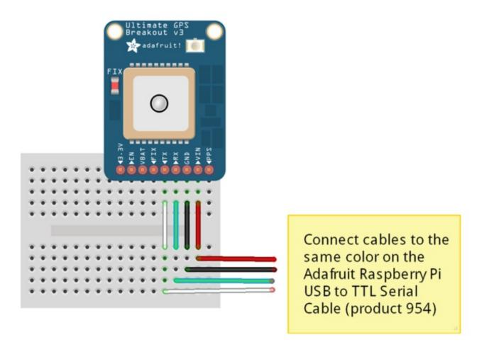
While the module on the Ultimate GPS Breakout has an exceptionally sensitive antenna and may work indoors as is, you may want to pick up an external GPS
